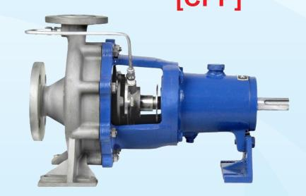
"Kemflow" Series PPF pumps are "Centrifugal Process Pumps" in Back Pull-out Construction, Horizontal, Foot Mounted, Single stage, End suction and Top Centerline Discharge confirming to DIN 24256 / ISO 2858, standards and in general confirming to API 610 as well.
